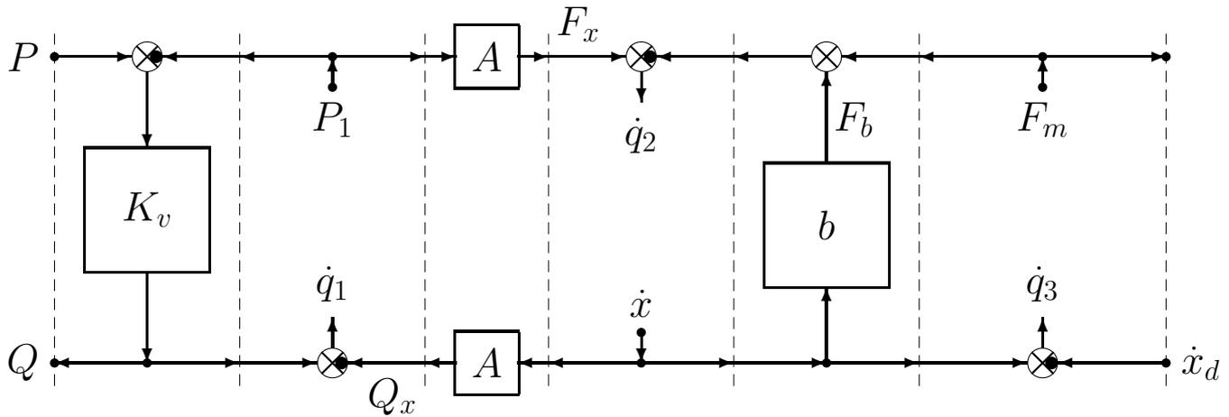
$$\mathbf{L} \dot{\mathbf{x}} = \dot{\mathbf{q}} = \begin{bmatrix} \dot{q}_1 \\ \dot{q}_3 \\ \dot{q}_3 \end{bmatrix} = \underbrace{\begin{bmatrix} -K_v & -A & 0 \\ A & -b & -1 \\ 0 & 1 & 0 \end{bmatrix}}_{\mathbf{A}} \underbrace{\begin{bmatrix} P_1 \\ \dot{x} \\ F_m \end{bmatrix}}_{\mathbf{x}} + \underbrace{\begin{bmatrix} K_v & 0 \\ 0 & 0 \\ 0 & -1 \end{bmatrix}}_{\mathbf{B}} \underbrace{\begin{bmatrix} P \\ \dot{x}_d \end{bmatrix}}_{\mathbf{u}}$$
