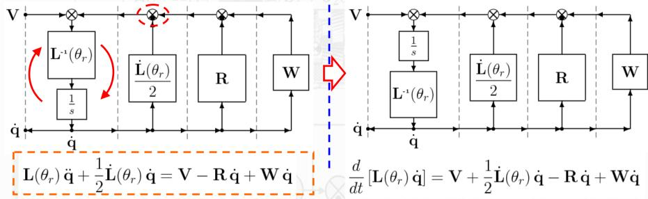
The dynamic equations can be easily interpreted from a "power" point of view.
