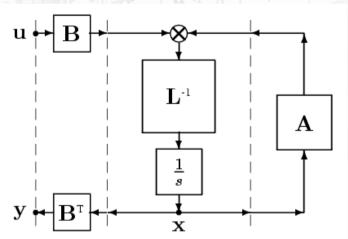
A "power" state space description of the DC motor with hydraulic pump:
