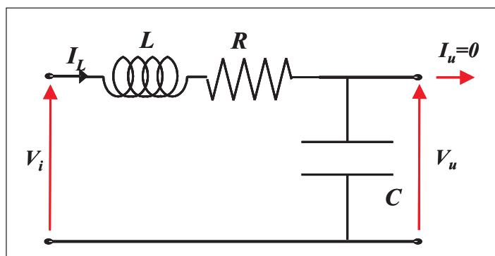
$$G(s) = \frac{V_u(s)}{V_i(s)} = \frac{\frac{1}{Cs}}{Ls + R + \frac{1}{Cs}} = \frac{\frac{1}{C}}{Ls^2 + Rs + \frac{1}{C}}$$
